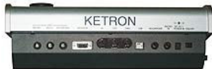
FIG. 2: All of the Midjay's inputs and outputs are on the instrument's sides and rear and recessed underneath its control surface.
